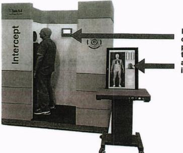
Intercept's built-in camera ensures a positive match between the person and their scanned image.
